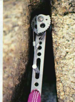
▲ A well placed Friend in a slight “down and out” flare. Though originally designed for parallel or slightly flared cracks, their sophisticated design (which evolved from 1972-1978) yields a device that will hold in flares up to 20° (depending on rock type).
