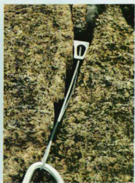
▲ This Rock™ placement, and the thousands like it that have held falls over the past 12 years, is testimony to the fact that climbing gear is seldom subjected to forces greater than 1000 kg (2200 lb.). We know this, first of all, because a UIAA labelled rope can not allow impact force of higher than 1100 kg and, secondly, although most Rocks now carry a 1200+ kg cable, for years they were specified at 1000 kg and we have never seen one broken in a fall. Thus, it seems apparent that above 1000 kg there is a certain level of needed redundancy in the strength of these nuts and most other climbing equipment.
